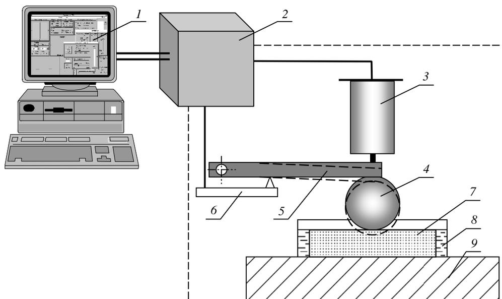
Fig. 1. Schematic diagram of the instrument for cartilage microindentation: 1 – a host computer; 2 – control electronic unit; 3 – an electromagnet for loading the indenter; 4 – spherical indenter; 5 – an arm for the indenter supporting; 6 – a piezoresistive AFM probe; 7 – sample; 8 – liquid medium; 9 – lifting platform
