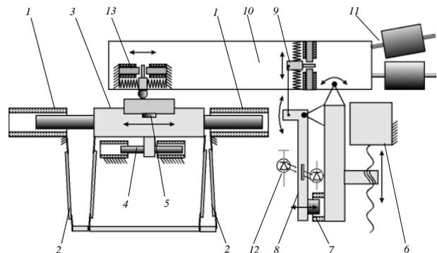
Figure 3: Precision tribometer scheme: 1 – drive electromagnets; 2 – flexible guides; 3 – holder table for specimens; 4 – position transducer; 5 – acoustic emission transducer; 6 – stepping drive; 7 – electromagnet of loading unit; 8 – lever; 9 – loading transducer; 10 – head; 11 – balancing weights; 12 – optocoupler; 13 – friction force transducer
