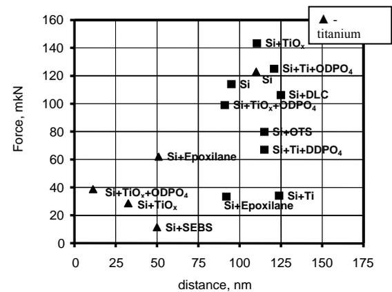
Figure 6: Test values of action radius of attraction force and magnitude of the maximal attraction force for various indenters
