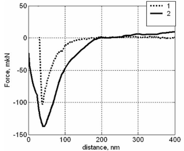
Figure 5: Experimental dependence force - distance. 1 – interaction of silicon ball and Si+TiO<sub>x</sub>+ODPO<sub>4</sub>. 2 – interaction between titanium ball and silicon plate.
