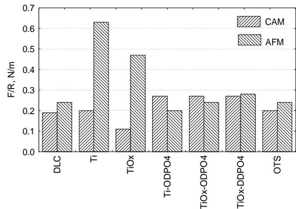
Figure 7: Adhesion (CAM) and pull-of forces (AFM) of the specimens.
