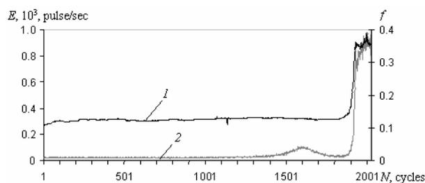
Figure 8: Friction coefficient  $f$  (1) and AE counting rate  $E$  (2) vs. number of test cycles  $N$ . Normal load  $P = 300$  mN; sliding velocity  $v = 4$  mm/s, track length  $S = 3$  mm
