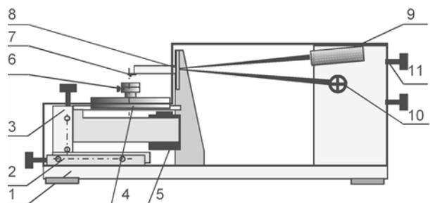
Figure 4: General scheme of rotary/reciprocating microtribometer: 1 – base plate; 2 – horizontal positioning plate; 3 – system of vertical positioning; 4 – rotary or linear electromagnetic motor; 5 – electromagnet; 6 – sample stage; 7 – ball holder; 8 – spring suspension; 9 – laser; 10 – four-quadrant photo detector; 11 – tuning screws.
