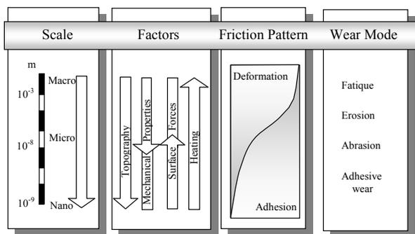
Figure 1: Combination of factors effecting friction and wear
